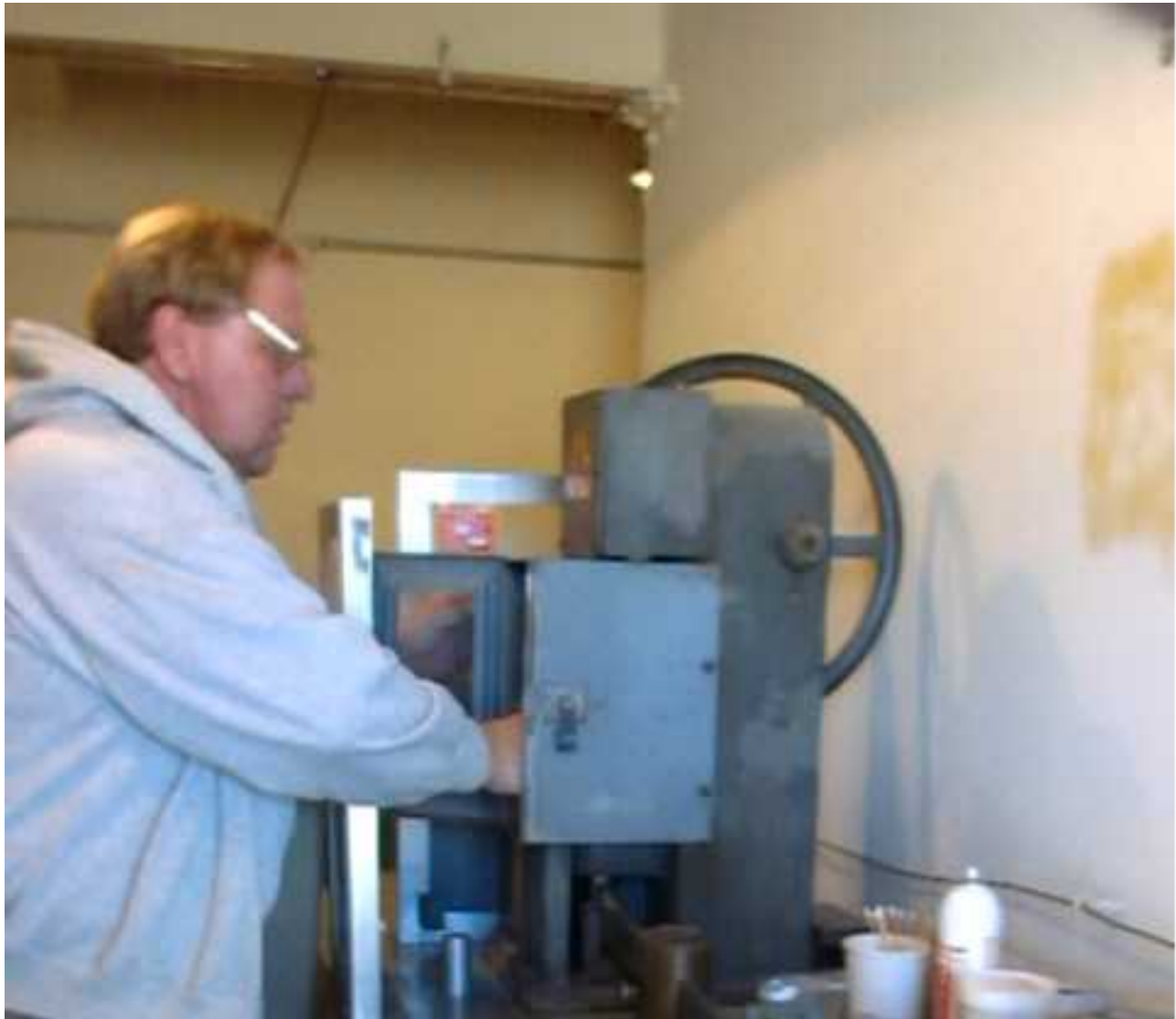
Figure 4 - Lead Free Primer Pressing Operation
