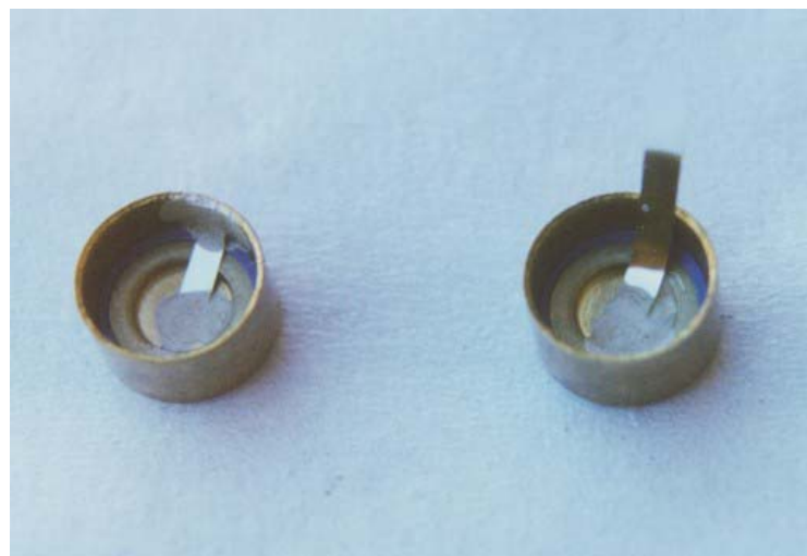
Figure 2 – Alternate (Exploding Foil) Electric Primer Configuration
