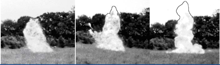
Figure 5. The fireballs from 1-litre tests .The left-hand photo is from the non-directional fuel explosion (as per Figure 1). The middle photo is from the directional fuel explosion (as per Figure 2). The right-hand photo is from the 'compression tube' firing. The black outlines, were added before rendering the photos in greyscale, to better identify the extent of the fireballs.
